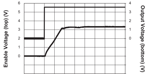
LDO Turn-On Time from Enable
